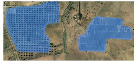
Left: a dual axis facility. Right: a static facility. The static facility has a notably higher ground coverage ratio (GCR) and therefore greater capacity. This is not directly captured however. GCR - and by extension capacity - estimates for both of these facilities are based on the size of the facility and country of origin.
